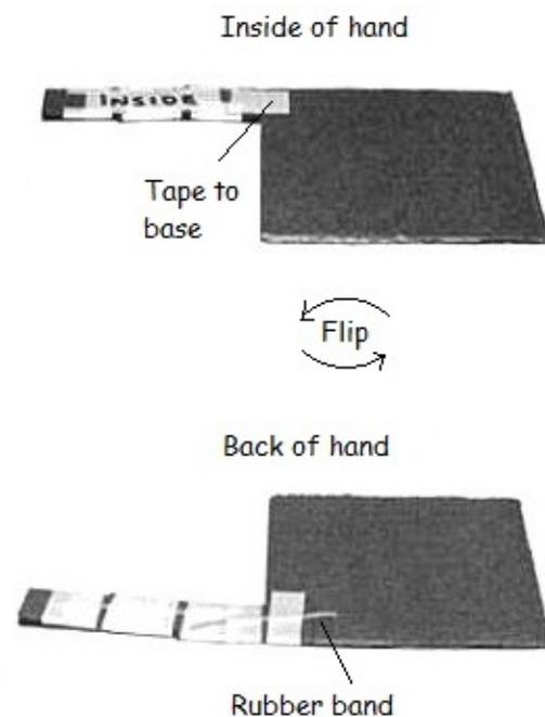
**Procedure:** Tape the finger (inside up) onto the palm. Turn the hand over and fasten the last finger joint to the palm using the same method as above.
