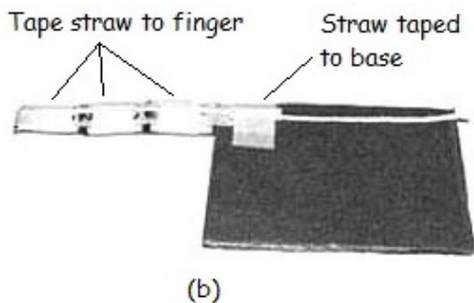
**Procedure:** Cut a piece of string about 35 cm long and tape one end firmly over the end of the finger. Cut four pieces of straw each about 2 cm long and thread them onto the string. Tape three of the straws in the middle of each of the finger sections. Tape the last straw to the palm as shown.
