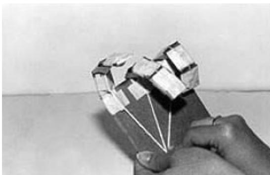
**Procedure:** Repeat the steps above for the last two fingers. When finished, operate the hand by pulling the strings. You should be able to pick up empty soda cans and other light objects with your hand.
